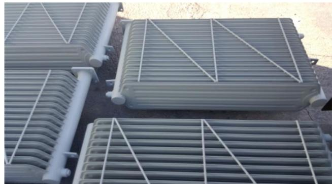
Transformer components (control box cases, radiators): Topcoat applied
