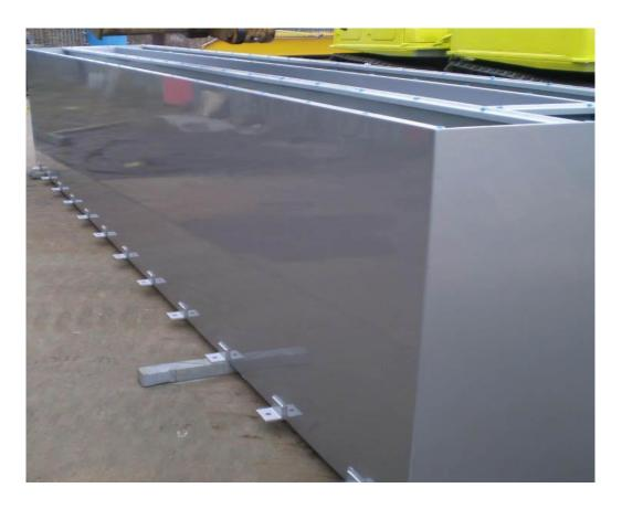
The crash barriers have cross-sectional stiffeners welded into place by friction welding for maximum strength.
